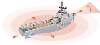
Auto position mode automatically maintains the required position and heading.
