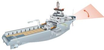
Auto heading mode automatically maintains the required heading.
