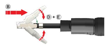
Position the chuck onto the RJ45.
