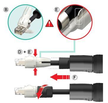
F Slide the sleeve onto the chuck thread and tigthen it.
