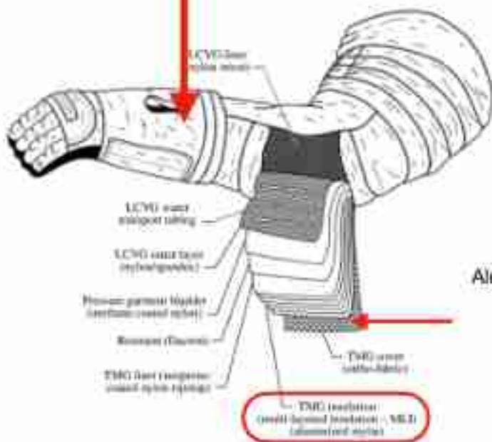
Aluminized mylar laminated to a nylon ripstop material that forms a radiant barrier in spacesuits.
