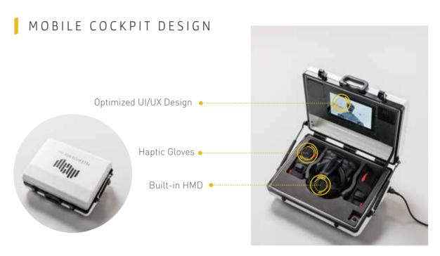
Conventional robot control interfaces are bulky, non-mobile and requires long setup time. At Telexistence Inc, we want to provide freedom and best mobility experience to our valued customers by introducing a carry on luggage type compact all-in-one cockpit package with built-in HMD, body trackers, data gloves and haptic devices. TX cockpit is airplane-approved carry-on size and weight so that our customers can access their remote robots from anywhere in the world.
