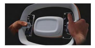
Valeo's steering wheel switches are designed to enhance driving control and comfort. These advanced switches make it possible to manage all assistance, automated driving and infotainment functions without taking your hands off the wheel or your eyes off the road.
